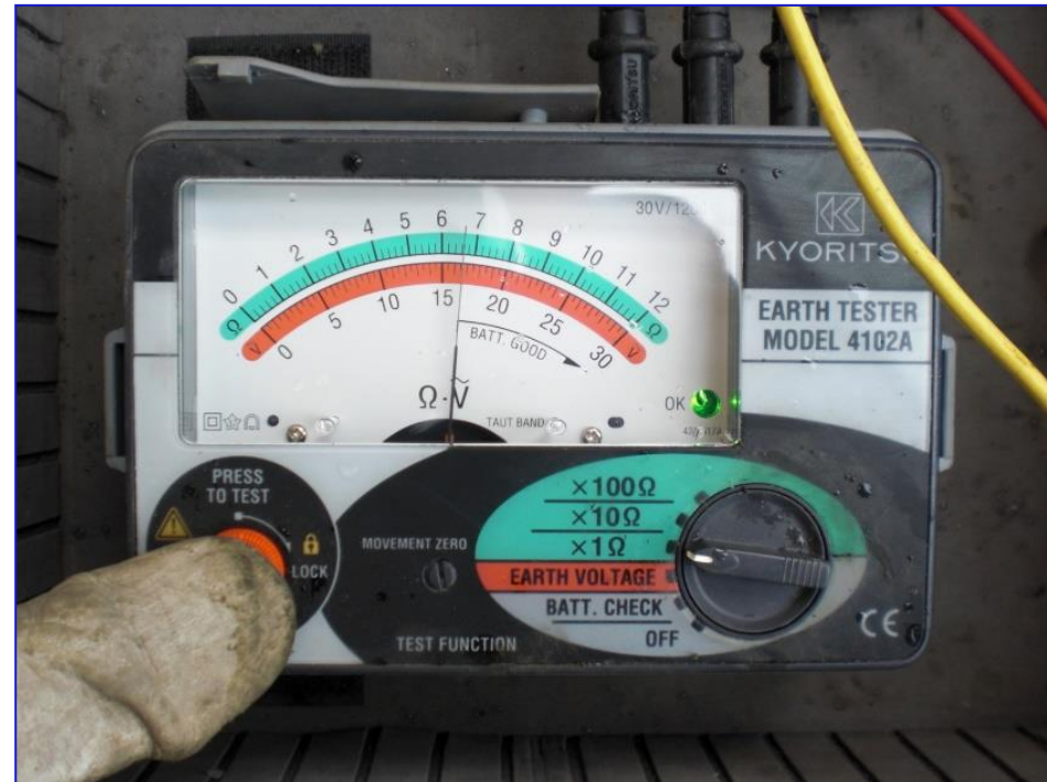
Resistance R = 6.6 \Omega on \times 1 \Omega scale
