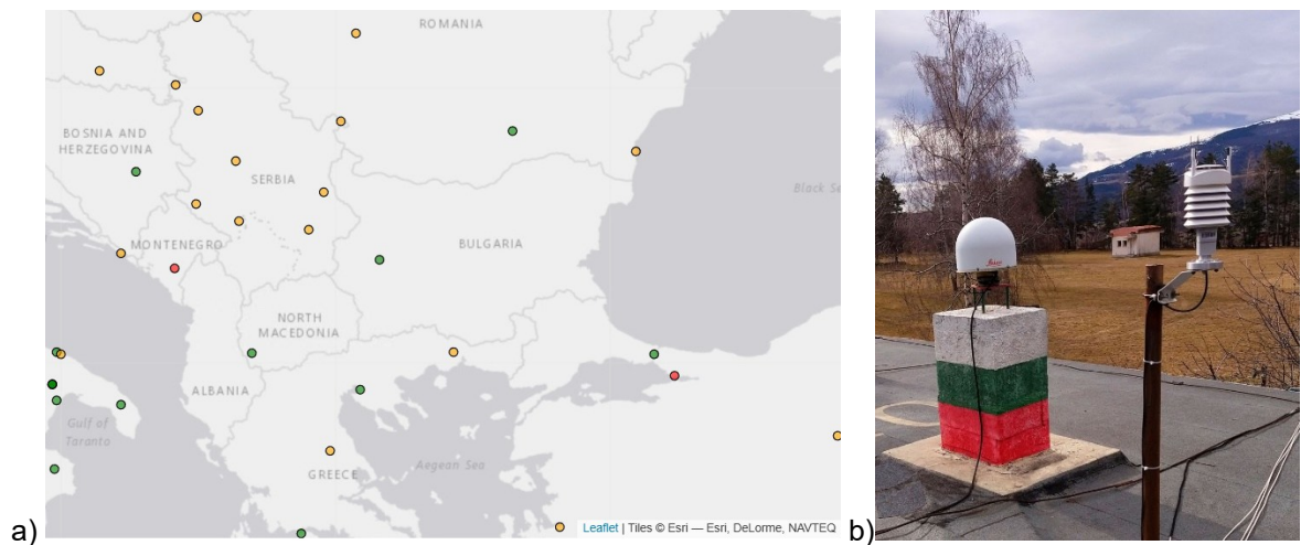
Figure 1 (a, b). a - EUREF EPN coverage in SE Europe. Stations in green are providing daily, hourly & real-time data; stations in orange - daily & hourly data; stations in red - only daily data; b – the EPN station SOFI , located near Sofia.
