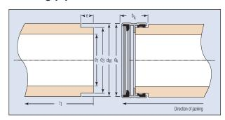
The coupling consists of glass fibre reinforced polypropylene. Vitrified clay DN 150 jacking pipes can be connected to Steinzeug | Keramo standard pipes directly with the jacking coupling or via the metal banded M couplings (spigot-spigot).
